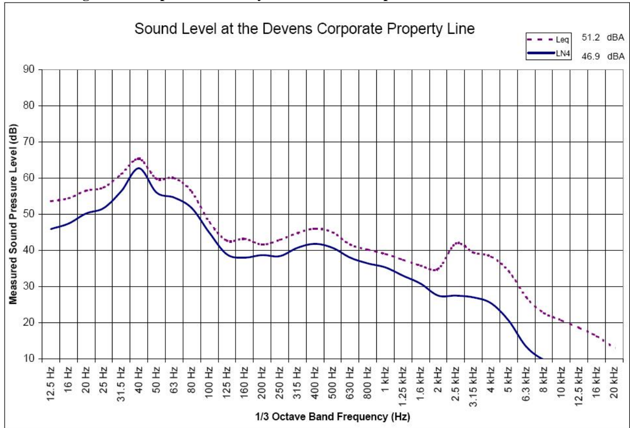
Figure 2: Graphical Summary of the Measured Spectrum at the Evergreen Solar Equipment
