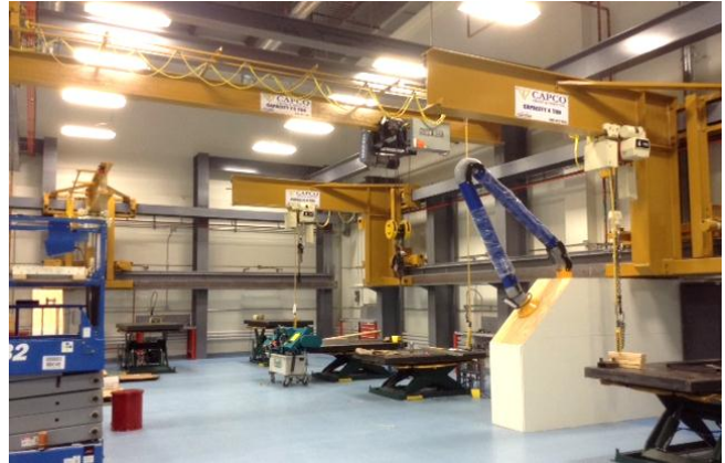
Work room: Testing hoists and beams that will transport molds into place.
