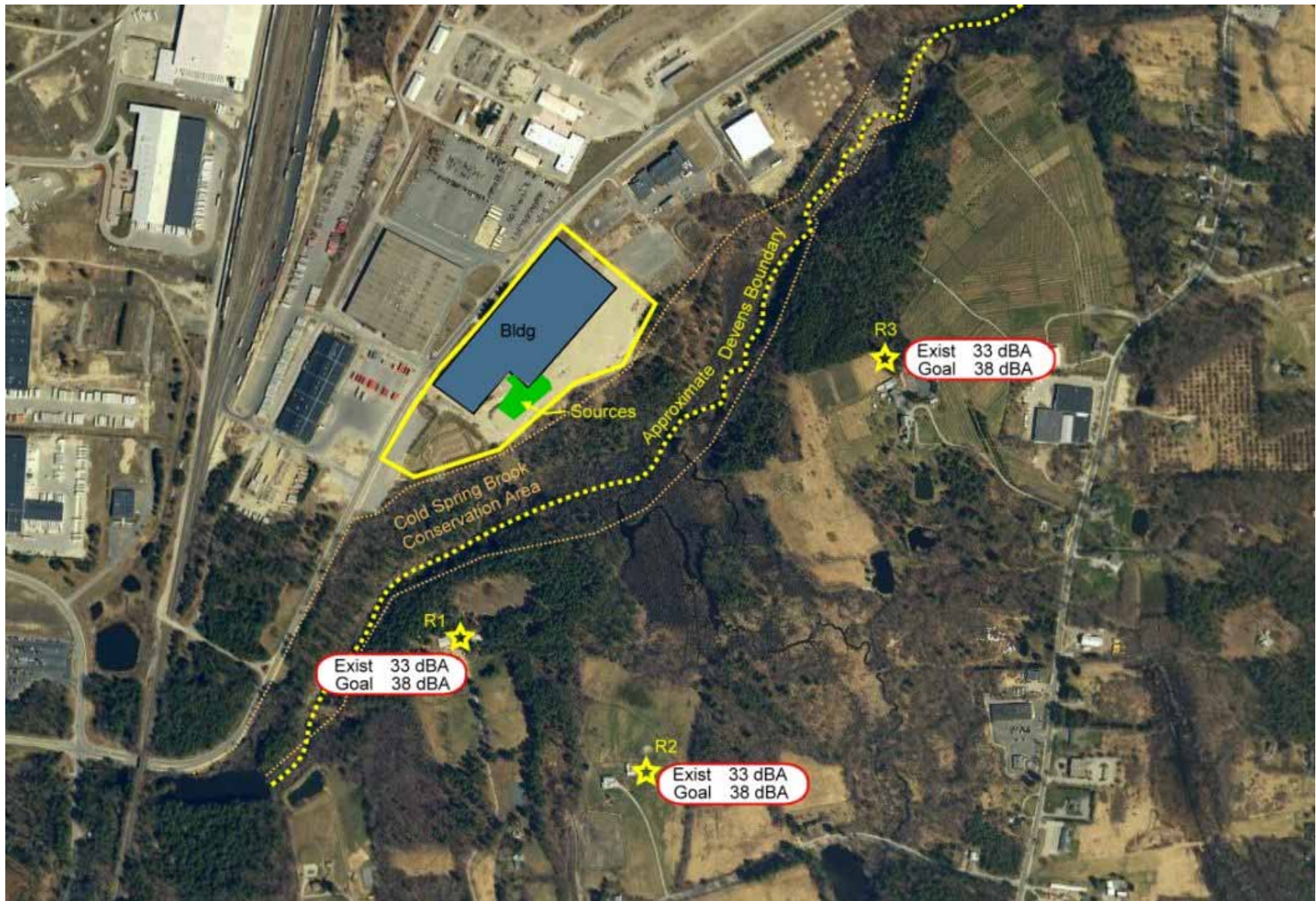
Figure 1: Project Area Showing Nearest Receptors and Summary of Project Baseline and Regulatory Limits
