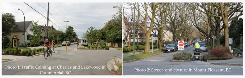
Green and Complete Streets Components: Photo 1 has a traffic calming diverter, discouraging through traffic on the neighborhood bike lane. Photo 2 has a street-end closure allowing the neighborhood bikes and pedestrians through.
