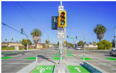
Green and Complete Streets Components: Protected bike lanes, bicycle signals are coordinated with traffic signals, crossbikes/crosswalks, and higher curb between street and bike facility.
